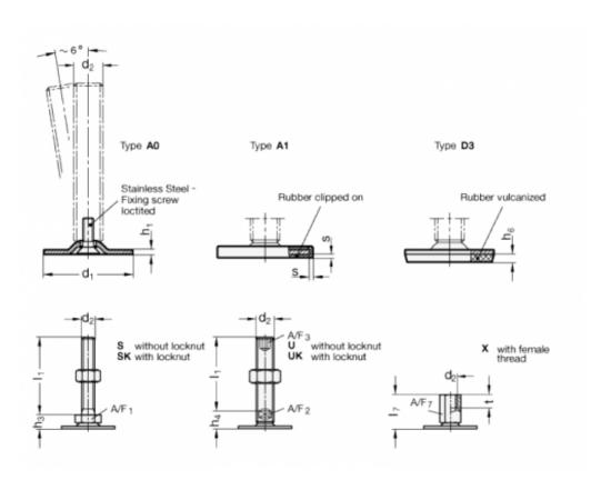
$\begin{array}{lll} A/F1 = 17 \\ d1 &= 60 \\ d2 &= M8 \\ h1 &= 2.5 \\ h3 &= 11 \\ h6 &= \\ l1 &= 63 \\ s &= 1.5 \end{array}$
